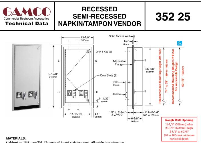
**Cabinet** — 18-8, type-304, 22-gauge (0.8mm) stainless steel, All-welded construction,
